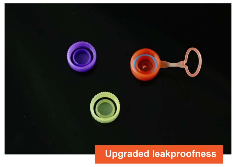
The flexible O-ring in the screw cap ensures safe closure of the micro spiral vial and a sound sealing effect. It meets ADR & IATA standards, and is free of liquid leakage during negative pressure 0.95bar test.
